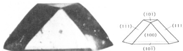
Figure 1. Photograph of a typical crystal of I (approximately 0.5 cm along the longest edge). On the right is a schematic diagram of the crystal showing Miller index assignments of the prominent faces.
